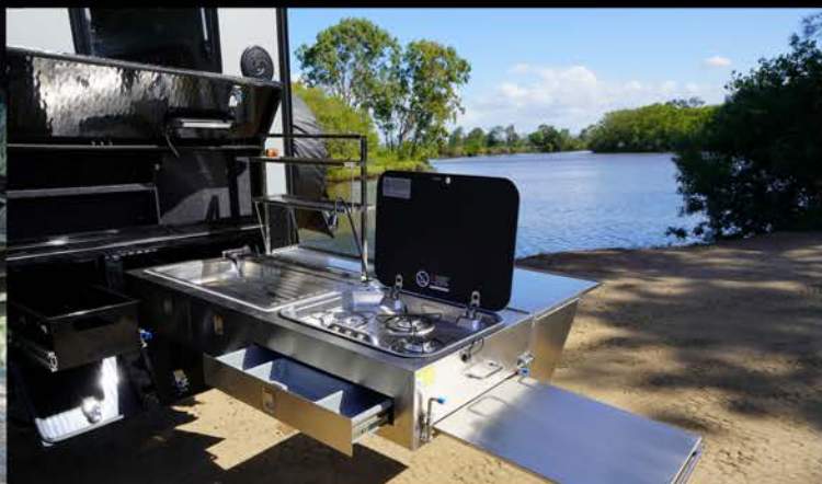
Slide out stainless steel kitchen with cutlery drawer, utility drawers, electric pump, hot/cold tap, large sink & AGA approved multi burner stove with wind break. Drainage rack, rear prep bench & large slide out kitchen preparation bench. Multiple storage compartments
