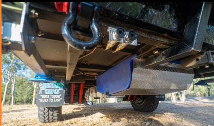
Water storage: 2 x 120L Foodgrade poly water tanks. 12.5L per min 12V Electric Pump. Water tank guards, water gauge.
